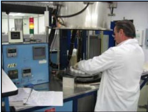
**INTA Technologies utilizes atmosphere controlled furnaces**
